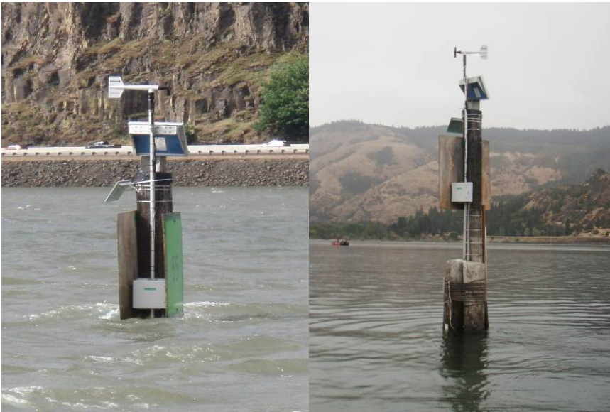
Figure 14. Klickitat River delta Daybeacon 55 site at high (left) and low Bonneville Pool stage (right). Photos of stage levels were taken on June 1, 2011 and September 26, 2011, respectively.
